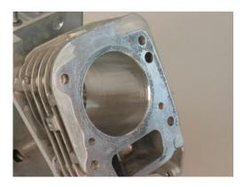
Cylinder Block: the largest single part of an engine; the main mass of metal where the cylinders are bored or placed.
