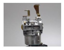
**Carburetor:** a device for automatically mixing fuel in the proper proportion with air to produce a combustible gas.
