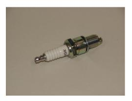
**Spark Plug:** a device inserted into the combustion chamber of an engine that contains an insulated control electrode for conducting current.
