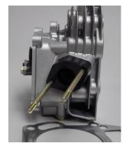
**Cylinder Head:** a detachable portion of an engine fastened securely to the cylinder block that contains all or part of the combustion chamber.
