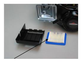
**Air Cleaner:** a device that filters the air that is mixed with the fuel in the engine.
