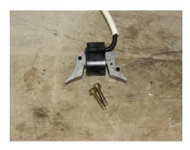
**Armature:** a part consisting of coils of wire around an iron core that induces an electric current when it is rotated in a magnetic field.
