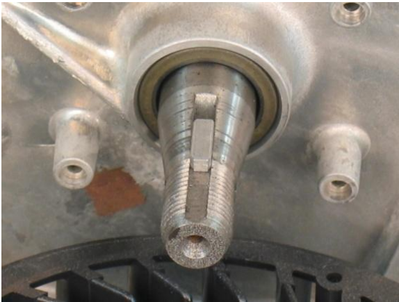
Flywheel Key: a device that holds the flywheel in place.
