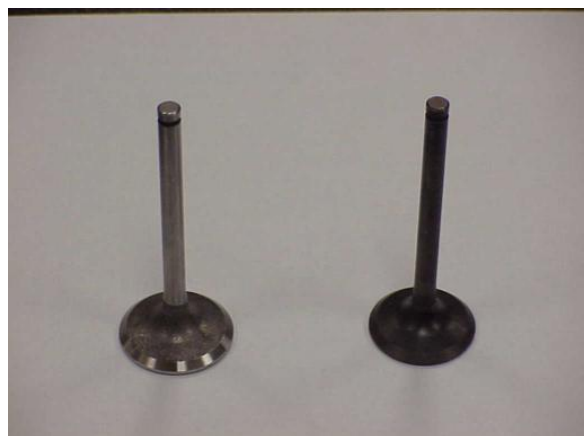
Exhaust Valve: a valve that permits the remains of the burned fuel to leave the combustion chamber.
